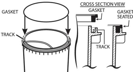
**Model 16000 O-RING** seats on top step of outer flange. First position O-ring onto step as shown then cover all exposed surface of O-ring with silicone grease (supplied in small packet).
