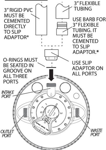
**WHEN USING RIGID PVC PIPING, 3" UNION CONNECTIONS\* MUST BE USED ON ALL 3 LINES FOR ABILITY TO DISCONNECT AND REMOVE LID.**
