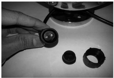
To connect additional LED lights to one ballast join the male end of the additional light to the Female end of the first light. Observe the following steps to connect additional LED Lights
