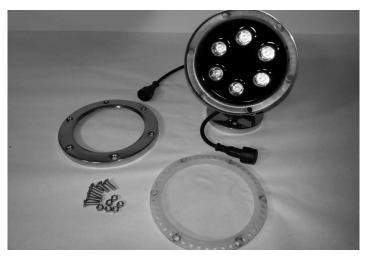
**MAINTENANCE:** Using an Alan wrench take off the screws and nuts. Remove the steel top ring. Take off the rubber ring and the glass. Clean any moisture or dirt. Replace the rubber ring and the glass cover. Make sure to align the holes in the rubber ring with the screw holes. Replace the top ring and install the screws
