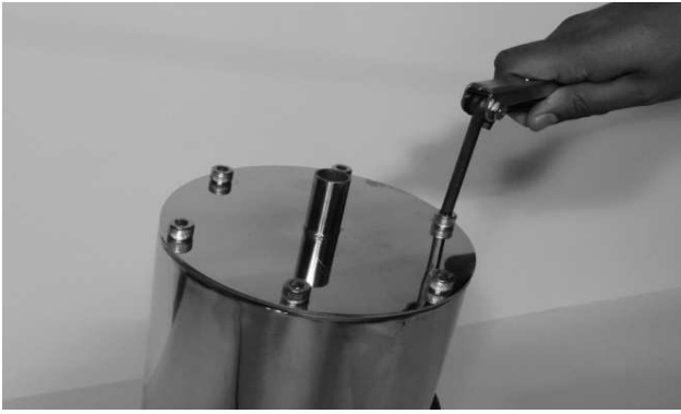
Using an Alan wrench remove the screws
