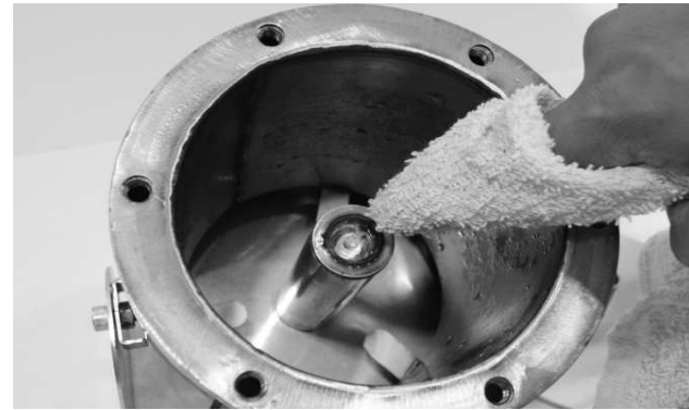
Using a soft cloth clean the LED Lens
