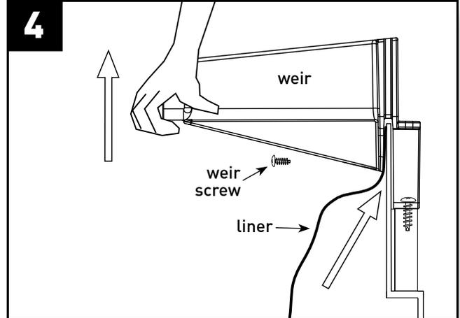
**4** Gently lift weir front. Then slide liner between filter and bottom weir supports. Carefully secure the liner to the Livingponds Filter<sup>™</sup> to maintain a water-tight transition between the filter and waterfall.
