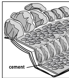
A smooth bottom pond makes waste removal easy and allows the pond to operate for decades without draining. The pond is able to achieve a stable natural balance that only comes with age. If desired, cement lined rocks can be run up the pond sides as well.
