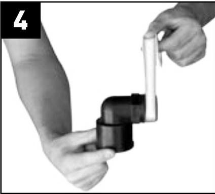
4 Put teflon tape onto 90° elbow.
