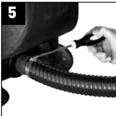
5 Attach hose and tighten clamp.
