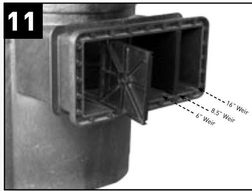
Insert weir dividers into Skimmerfilter™ neck. Use the tracks which correspond with the faceplate provided with your kit, as shown in the picture above. (8' x 11' pond uses innermost tracks / 11' x 16' and 16' x 21' use middle tracks)
