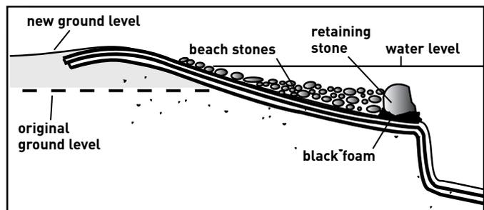
At the entry point of your pond, create a gradual sloping shelf. Place larger retaining stones at the edge of the shelf, 6" - 12" below water level. Secure the coping stones and fill the gaps between rocks with black foam. Backfill the area with 2" - 4" smooth river stones at least 2' out of the pond. To prevent water loss due to capillary action in the soil at the pond edge, extend the pond liner so it extends at least 2' out of the pond.
