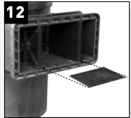
Push the weir door hinge tabs into notches on the weir dividers, using thumbs to hold tabs secure. Lay the door horizontal in the Skimmerfilter™ neck.
