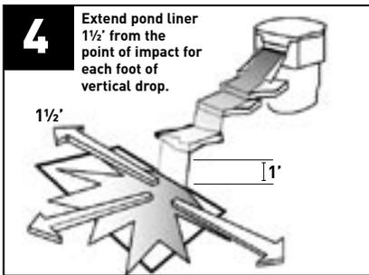
**4** Extend pond liner 1½' from the point of impact for each foot of vertical drop.
