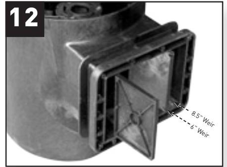
Insert weir dividers into Skimmerfilter™ neck. Use the tracks which correspond with the faceplate provided with your kit, as shown in the picture above. (6' x 10' pond uses innermost tracks)
