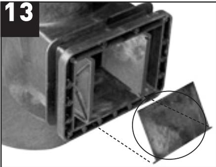
13 Push the weir door hinge tabs into notches on the weir dividers, using thumbs to hold tabs secure. Lay the door horizontal in the Skimmerfilter™ neck.
