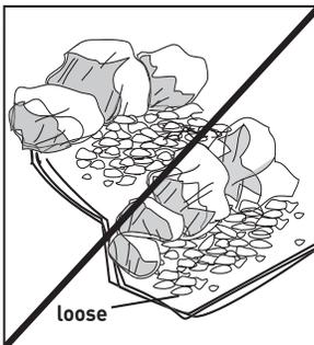
Loose rock traps debris, fosters anaerobic bacteria (which poses a threat to fish health) and can damage the pond liner. As debris accumulates, the only way to clean a loose rubble pond is by fully draining it, removing the fish and plants and then power washing the rocks.
