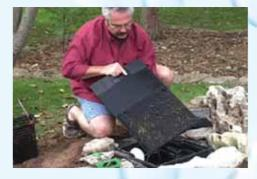
Slowly lift out the filter mat. Do this slowly and carefully to retain the most debris on the mat.
