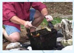
Empty the leaf basket on a weekly basis, more often if needed. In the Fall, skimmer may need to be cleaned daily. Leaf basket must stay clean to allow water into pump to prevent overheating the pump.
