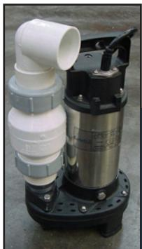
Your pond kit includes a check valve assembly which allows water to be pumped up to the filter but does not allow backflow from the filter to skimmer. Thread the check valve assembly into the pump discharge. Place the pump into the skimmer. If your check valve has a rubber boot, slide the boot over the flexible pvc pipe and tighten clamp. If your check valve has built in unions, glue the outlet onto the flexible pvc pipe.
