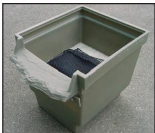
The mini AquaFalls installs differently than the other AquaFalls filters. The filter tub and stone lip are molded into one piece. The liner is held to the tub, under the lip, by a plastic strip and five bolts. Place a bead of silicone over the bolt inserts, hold up liner, then attach plastic strip to tub with bolts and washers.
