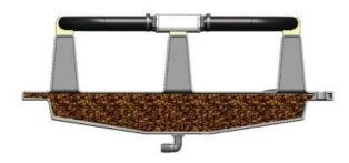
3. Install vent plug once base is completely full.
