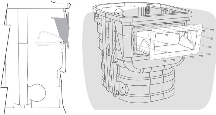
Use your fingers to hold the flange nut and a hand held screwdriver to tighten the screws. The serrations on the flange nut will grab the plastic enclosure once it makes contact, eliminating the need to use a wrench. Use caution when tightening the screws. The screws need only be snug for the silicone to make a seal.
